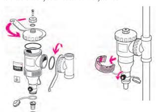
Debris which has been collected by the DirtmaglQ<sup>™</sup> needs to be removed using the blow down valve.
