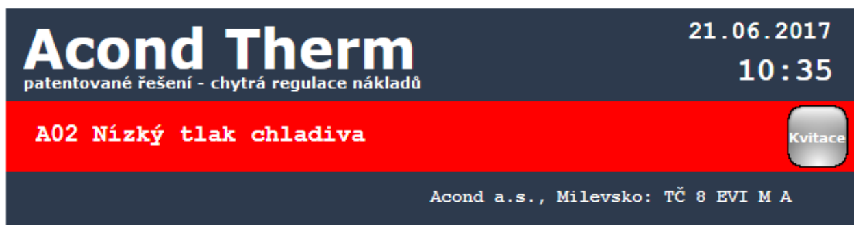
Figure 10 From the fault display on the web page
