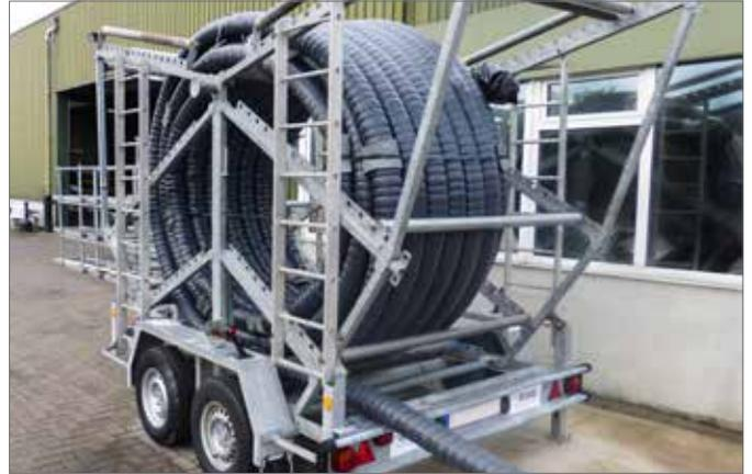
Fig. 7-30 Vertical mobile unwinding device
