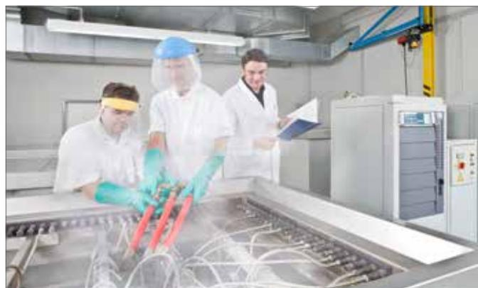
Fig. 6-18 The leak-tightness of the pipes is investigated during the long-term test
