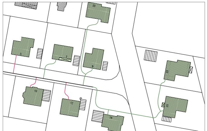
Fig. 6-6 Connecting different pipe systems
