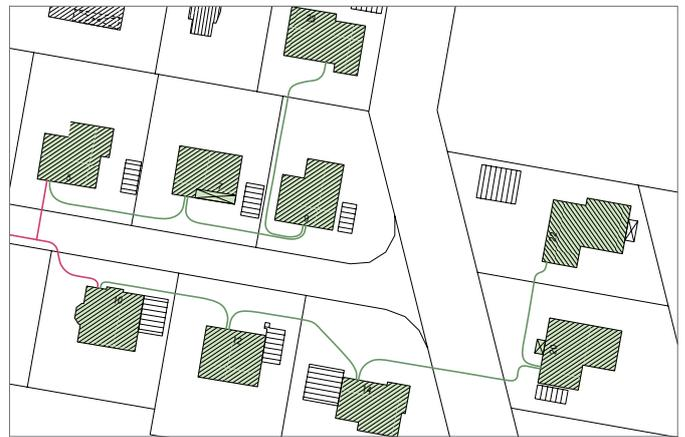
Fig. 6-5 „House-to-house“ line arrangement / building to building piping
