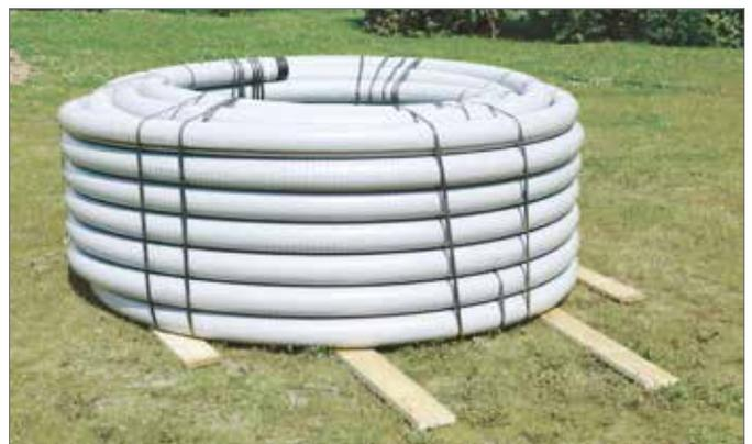
In the case of vertical storage objects in the outer jacket can be pressed into the relatively small supporting surface due to the weight pressure.
