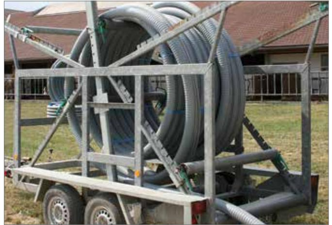
Fig. 7-6 Pipe uncoiling trailer
